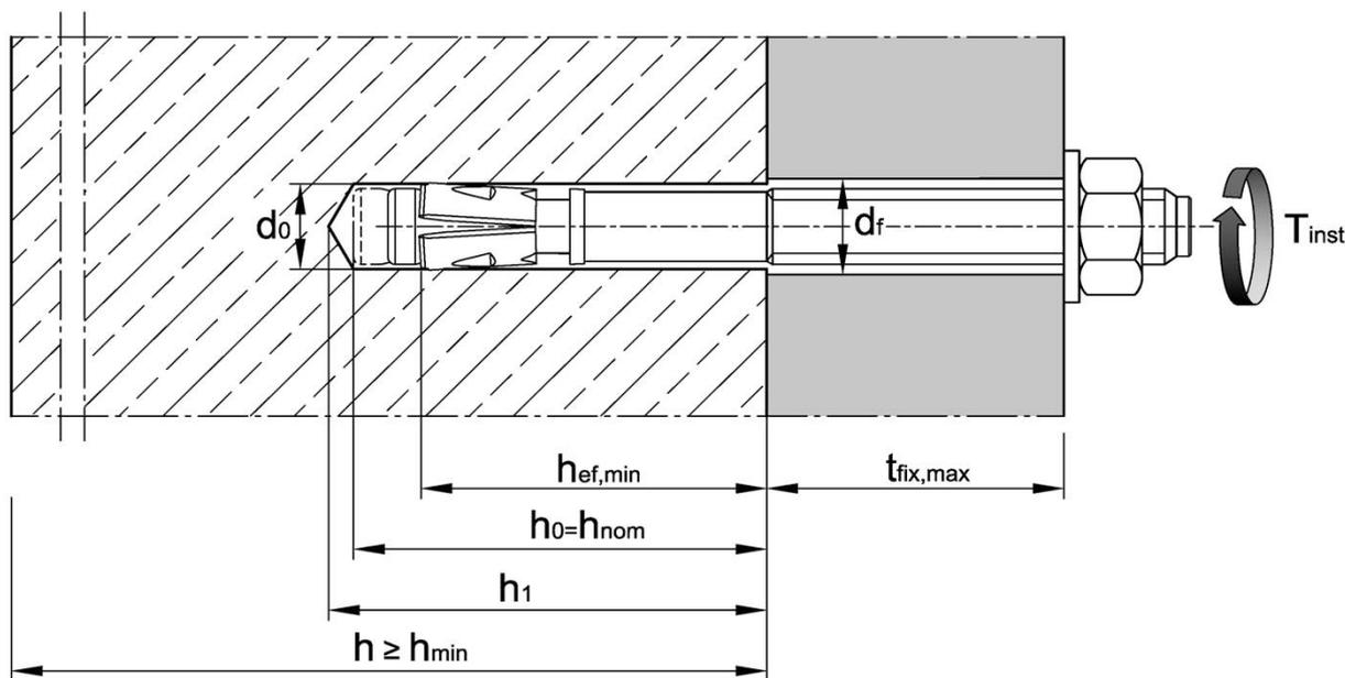
**Bolzenanker BZ3 / BZ3 A4 / BZ3 HCR**
