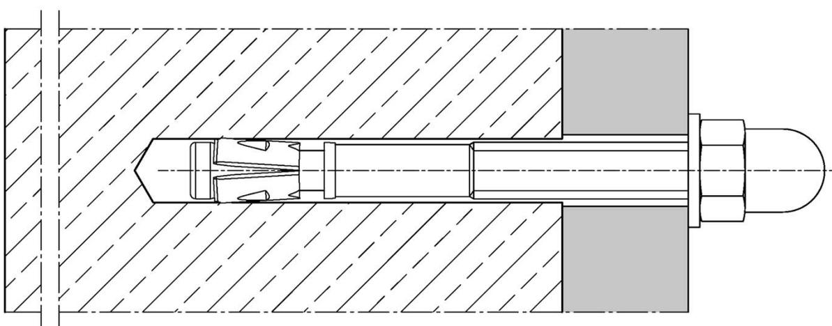
**Bolzenanker BZ3 / BZ3 A4 / BZ3 HCR**
